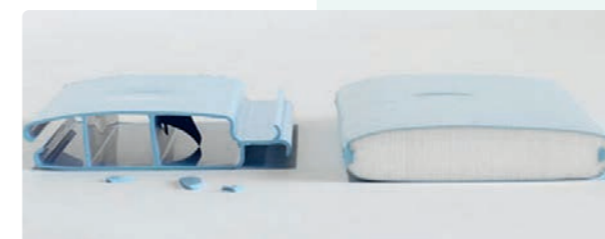
After the hail test, conducted by an external and independent laboratory. On the left: standard hollow slats On the right: Covrex® Classic slats
